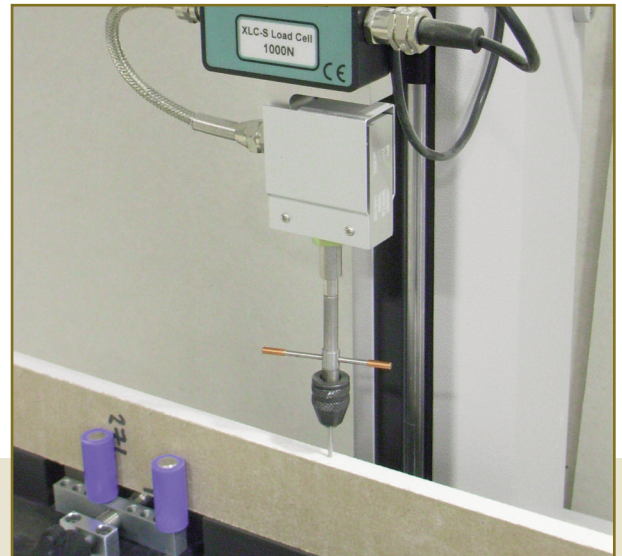
Probe shown attached to loadcell before being inserted into plasterboard sample
